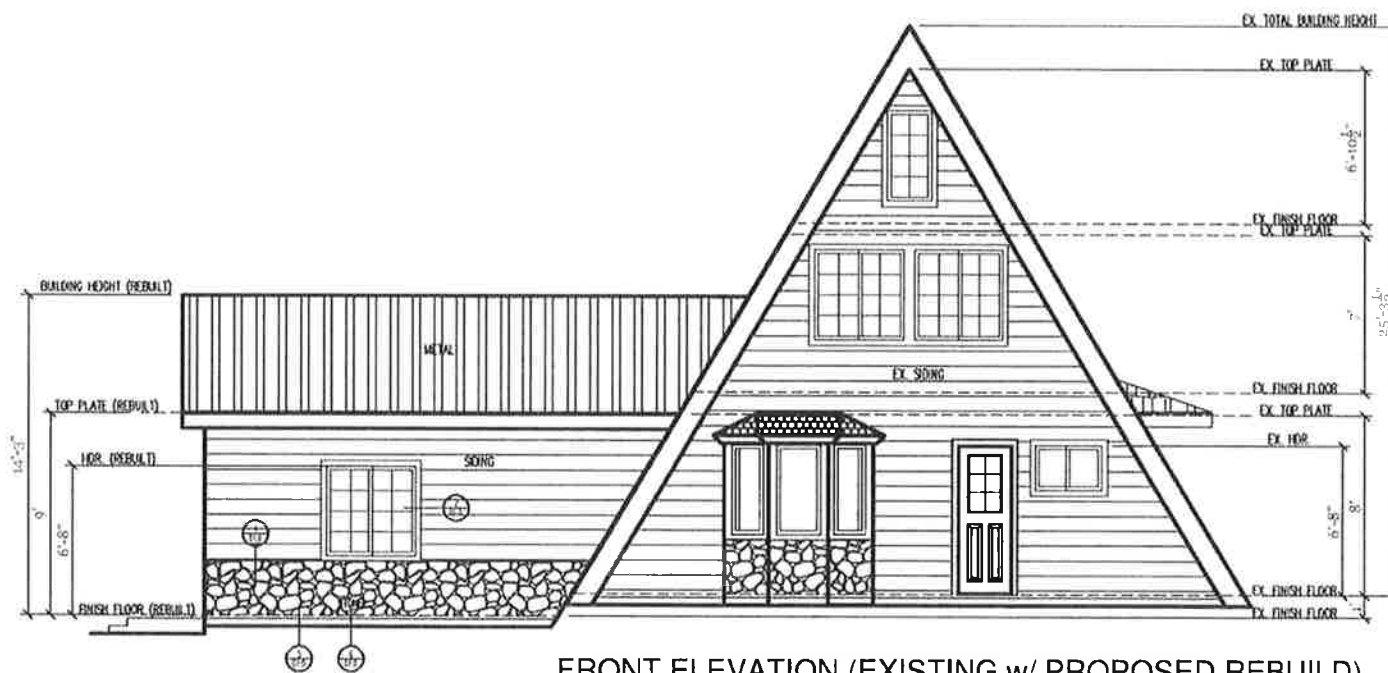
FRONT ELEVATION (EXISTING w/ PROPOSED REBUILD)
