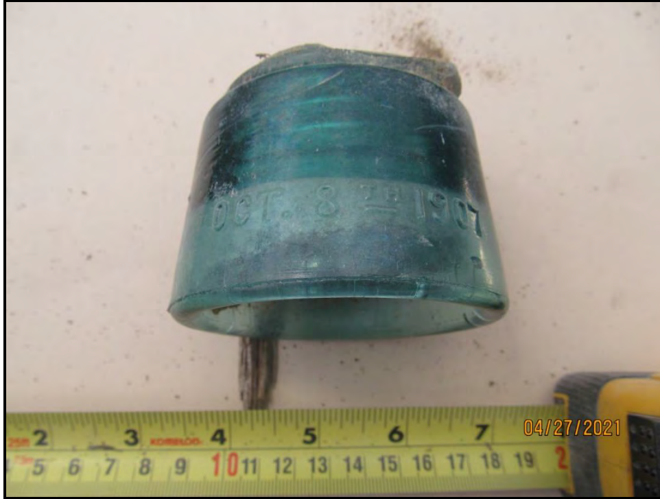
Log 1, Image 16, 26Wa12841, H-3 Broken aqua glass insulator "Patented Oct. 8th 1907," 3 3/16 by 2? in. tall (Profile) Praana II Washoe BESS/PSES Site Project, UTM Zone 11, 245898 E/ 4449393 N
