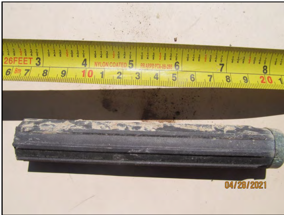
Log 1, Image 66, 26Wa12846, H-7 Vehicle battery core, 2 5/8 in. diam. By 4 1/8 in. length (Plan), Praana II Washoe BESS/PSES Site Project, UTM Zone 11, 245547 E/ 4449455 N
