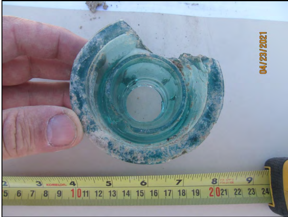
Log 1, Image 12, 26Wa12841, H-1 Aqua glass insulator "HEMINGRAY/ Pat 1907," 3 3/16 by 2 1/2 in. tall (Plan) Praana II Washoe BESS/PSES Site Project, UTM Zone 11, 246111 E/ 4449440 N
